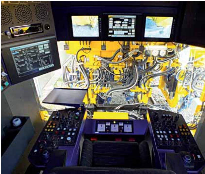
Work cabin of a universal tamping machine by Plasser & Theurer.
