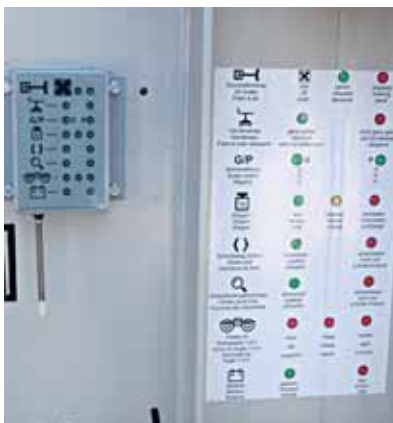
VTG box that signals situations right on the wagon to the operating personnel.
