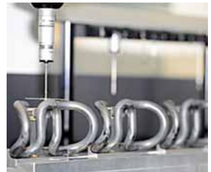
The W-shape of the elastic tension clamp of the key element provides the necessary safety.
