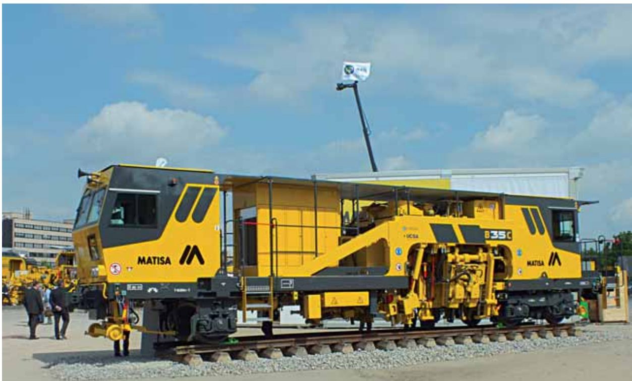
Insurgent universal tamping machine B 35 C by MATISA.
